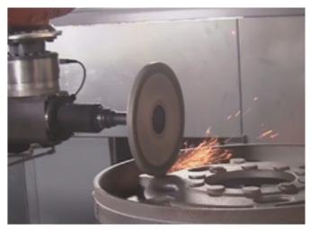
The workpiece is positioned on a CNC rotary table for machining within the production center. The rotary table axis is fully integrated into the robot control system.
