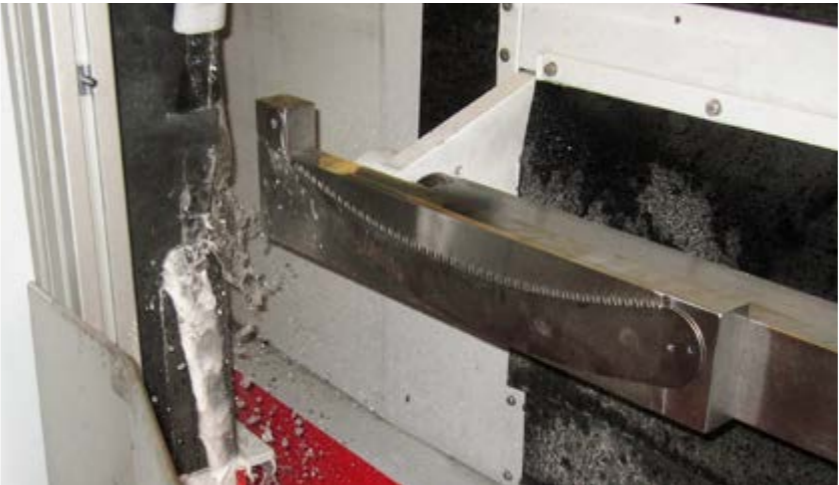
1 Conical relief grinding on saw blades with flat bevel grinding machine BG/NT
