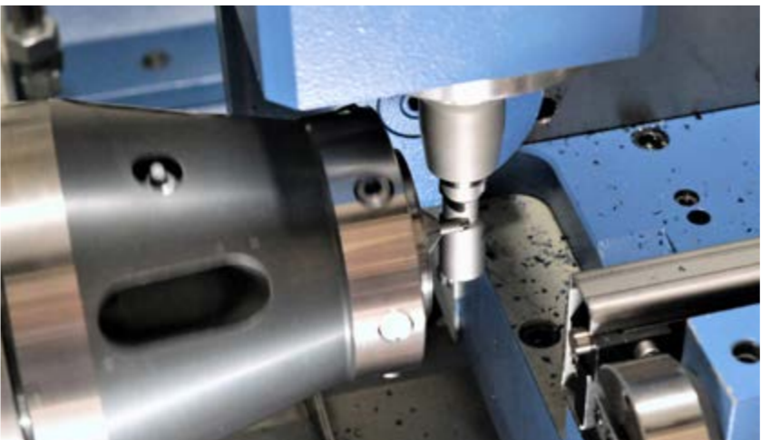
3 Profile generating of ball end screwdriver blade
