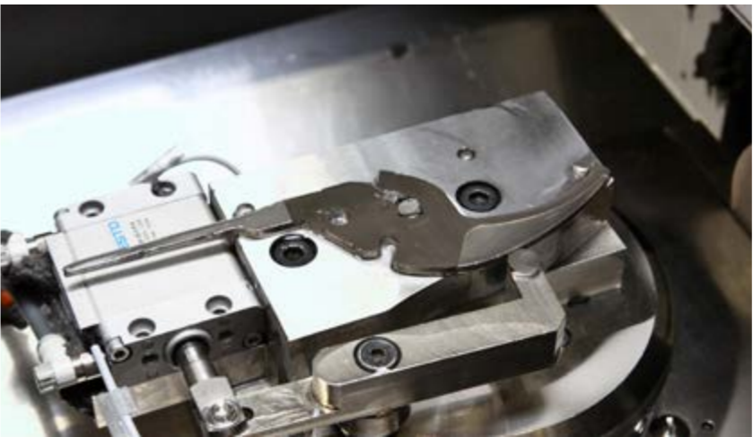
4 Flat grinding of garden shears with flat bevel grinding machine DG2/NT
