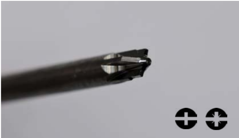
4 PlusMinus screwdriver blades after machining
