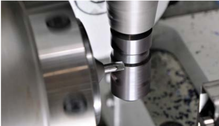
2 Profile generating of PlusMinus screwdriver blades
