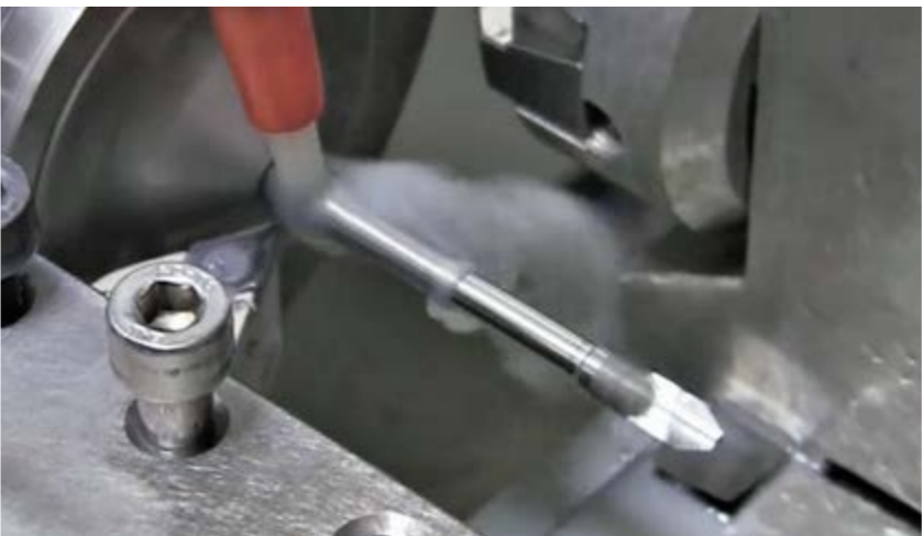
3 Long turning and ejection of the finished workpiece
