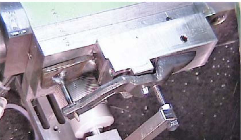
3 Surface grinding of plate shears with flat bevel grinding machine BG1/NT
