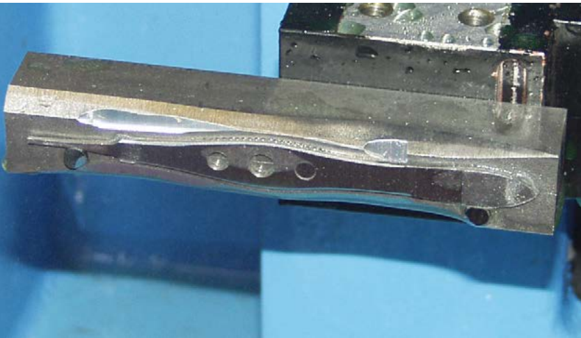
2 Grinding of the inside of eye tweezers
